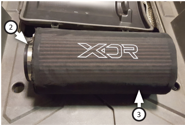
12. Fit pre filter wrap (3) over oiled air filter (2).
