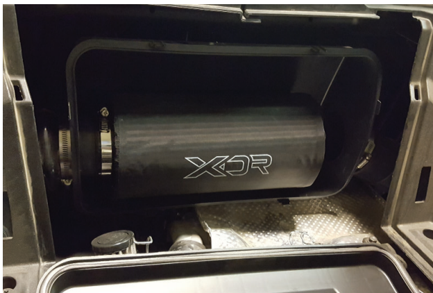
13. Install air filter assembly into airbox. Tighten clamps to secure it in place.
