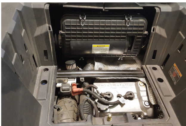
14. Inspect all installed components, securing connections and tightening all clamps to complete installation, then replace and latch air filter cover.
