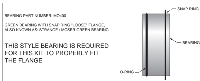
Figure 2. Loose Fit Bearing Configuration
