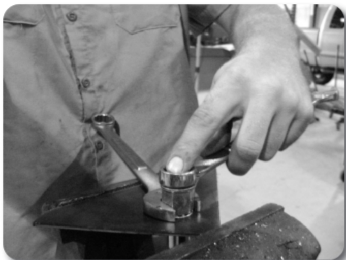
Figure 4 - 1/2" Rivet Nut shown
