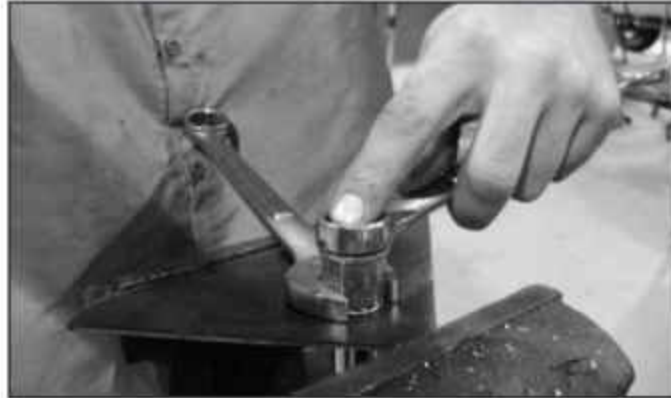
FIGURE 28 - 1/2" RIVET NUT SHOWN
