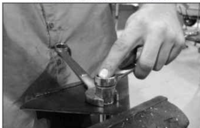
FIGURE 2 - 1/2" RIVET NUT SHOWN
