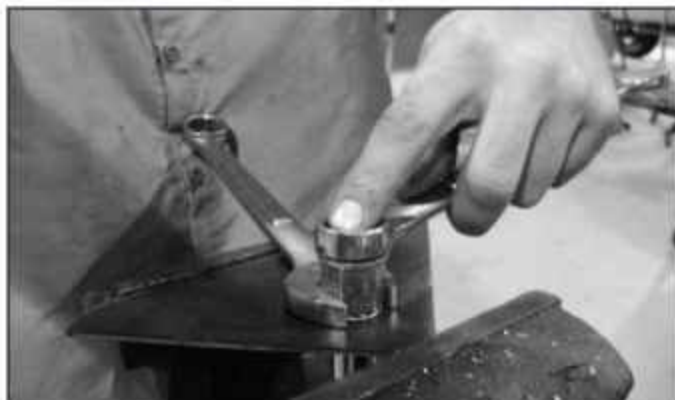
FIGURE 28 - 1/2" RIVET NUT SHOWN
