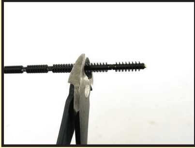
1- The linkage rod can be cut to length using side cuts.
