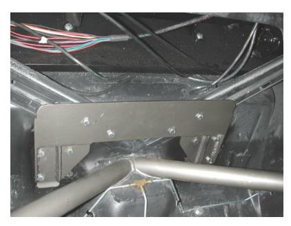
6. The inner support plate will bolt to the floor pan on the inside of the car using six 3/8" x 1" bolts, Nyloks and flat washers. The remaining 4 holes will need to be drill and will use 3/8" x 2 1/4" bolts, Nyloks and flat washers.
