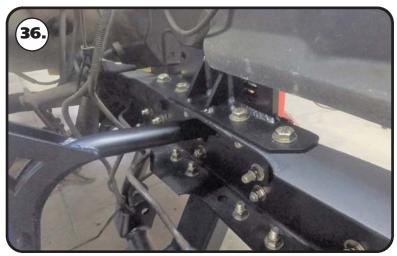
**36.** Install a 7/16" flat washer on each of (4) 7/16"- $14 \times 1/4$ " hex bolts. Insert a bolt/washer in each top (4) holes. Install a 7/16" flat washer and 7/16"-14 nylok nut on the threads of the bolts. Torque all 7/16" cradle hardware to 70 ft-lbs. Torque the 1/2" engine mount hardware to 75 ft-lbs.
