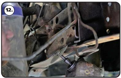
**12.** Cut the OEM steering box mount out of the frame by cutting it along the top and bottom frame rail.
