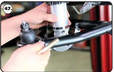
**47.** Swing the lower control arm up to the shock. While swinging the control arm up, insert the shock body into the shock mount of the control arm. Align the mounting holes with the through hole of the shock body.
