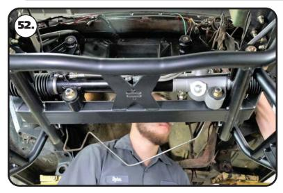
**52.** Install a M12 flat washer on a M12-1.75 x 170mm hex bolt. Insert the bolt/washer into the rack mount. Install a 1M12 flat washer & M12-1.75 nylok nut. Torque the hardware to 93 ft-lbs.
