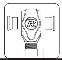
New R-Joints will be quite stiff (75-90 in/lbs breakaway torque) until they "break in" after a few miles of use. After the break in period they will move much more freely. Because the composite bearing race contains self lubricating ingredients, no additional lubrication is needed or desired. Any additional lubrication will only serve to attract more dirt and debris to the R-Joint and actually shorten its life.
