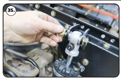
**35.** Insert the 1/2" ID Shock Bearing Spacers into the Bearing of the ShockWave/CoilOver. Install a 1/2" Flat Washer on a 1/2"-13 x 2 3/4" Bolts. Insert the top of the shock into the shock mount on the c-notch with the adjusting knob to the outside. Line up the holes and insert the bolt/washer. Install a 1/2" Flat Washer and 1/2"-13 Nylok Nut on the threads and tighten to 50 ftlbs.
