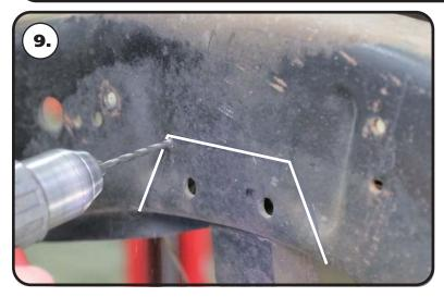
**8.** The corner holes will need to be drill with a 1/2" drill bit, but we recommend drilling the corner holes with a smaller drill bit first.
