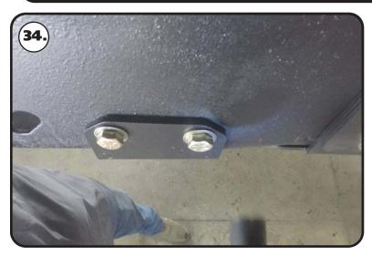
**34.** Install a 7/16" flat washer on each of (4) 7/16"-14 x 1 /4" hex bolts. Insert a bolt/washer in each of the (4) holes. Install a 7/16" flat washer and 7/16"-14 nylok nut on the threads of the bolts. Again, snug the hardware down, but do not torque the hardware at this time. Do this for both sides.
