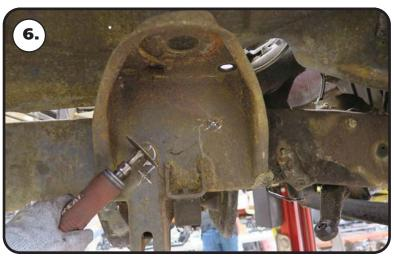
**6.** The OEM upper coil spring and I-beam mounts need be removed from the frame rail. This can be done by either drilling the rivets out or removing the rivet heads and driving them out. We remove the rivet heads by cutting a " + " in the head with a die grinder then we cut the head off with a hammer and chisel or with an air chisel. Once the head is removed, the rivet can be driven out with a hammer and punch.
