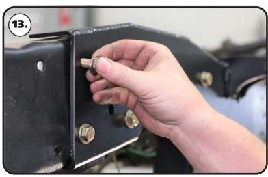
**13.** Install a 7/16" flat washer on each of (8) 7/16" x 1 1/4" bolts. This hardware gets installed in the sides of the c-notch. Install a 7/16" flat washer and 7/16" nylok nut on each bolt sticking through the frame. Tighten all of the c-notch side bolts. Tighten the hardware snuggly for the time being.
