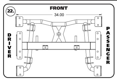
**22.** *Diagram 22* shows a top view of the cradle to illustrate which way it goes in the truck. The round tube of the cradle is to the front of the truck.
