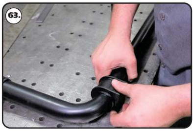
**63.** Open the sway bar bushing at the split and slip it onto the sway bar. Do this for both bushings.
