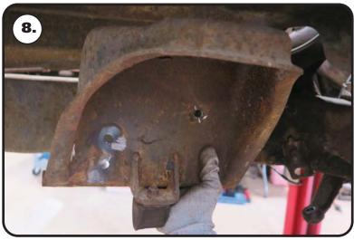
**8.** Remove the coil spring mount from the frame. Do this for both sides.
