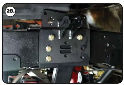
**28.** Install a 7/16" flat washer on a 7/16"-14 x 1 3/4" hex bolt. Insert the bolt in the top hole of the rear (3) bolt holes. This bolt will go through the upper control arm mount, cradle plate, & engine mount. Install a 7/16" flat washer and 7/16"-14 nylok nut on the threads of the bolt. DO NOT INSTALL A BOLT IN THE LOWER HOLE OF THE ENGINE MOUNT HOLE AT THIS TIME.
