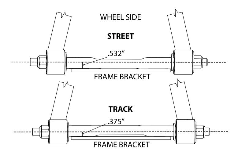
The cross shaft that is used in the upper control arms is offset. The offset combined with the caster slug option allows you to achieve the alignment setting you desire with minimal shims. To change the direction the lcon faces simply spin the cross shaft in the control arm.
