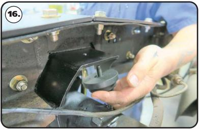
**16.** Install the bump stop using a 3/8"-16 x 1" socket head bolt, 3/8" flat washer, & 3/8"-16 nylok nut. Hold the bump stop with your hand and insert the bolt through the center of the bump stop. Line up the bolt of the bump with the drilled hole of the frame. Install a 3/8" flat washer and 3/8" nut on the threads of the bolt. Tighten to 60 **in-lbs**.
