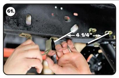
**61.** Use a tape measure to put a mark on the frame **4 1/4"** from the front edge of the cradle mount. Align the back edge of the sway bar mounting strap with the mark on the frame. Hold the mounting strap in the center of the frame and mark the center of each mounting hole. The mounting holes need to be marked on each frame rail.
