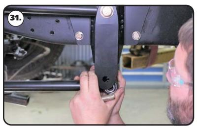
**31.** Insert (2) .625" ID x .740" long R-Joint spacers into the front R-Joint of each lower bar. The small diameter of the spacer goes into the R-joint. Insert the front lower bar R-Joint into the lower position of the frame mount.
