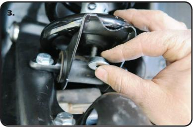
**3.** Using **(Figure 5)**, install a Stud Top Bushing Washer and Bushing on the Stud Top of the Shock. Insert the Shock through the OEM opening. Insert the studs into the openings in the lower mount. Using **(Figure 2)** as a reference, install a Bushing, Washer and Nut on each stud and tighten.
