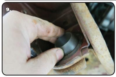
**9.** Refer to **(Figure 10)** for the Delrin Strut Rod Bushing assembly order. The Delrin Strut Rod Bushing will insert into the frame bushing hole with the rounded side of the bushing outward. A Bushing needs to be installed on both the front and rear side of the frame. With a Delrin Strut Rod Bushing on eaxh side of the frame, insert the INNER Sleeve in the Bushings. This will help hold them in place.
