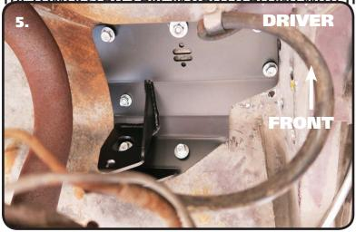
The biver upper shock wount repositions the top of the shock to behind the axle. The Mount nests in the car one way. Position the Mount in the car with the Shock attaching point to the rear and away from the frame. The outside edge of the mount will touch the frame with the front edge against a body seam. Using these points as a guide, the Mount will fit the contours of the body. With the Mount in position, use it to mark the 7 holes and drill them 5/16"
