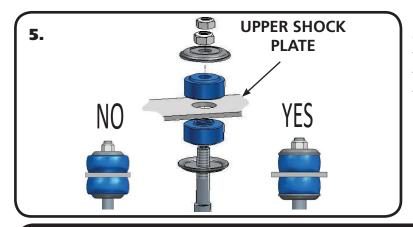
**5.** Install a Stud Top Bushing & Bushing Washer on the Shock. Install a 3/8"-24 Jam nut on the threads and tighten until the Bushings just start to bulge. Install a 2nd 3/8"-24 Jam Nut and tighten it against the 1st.
