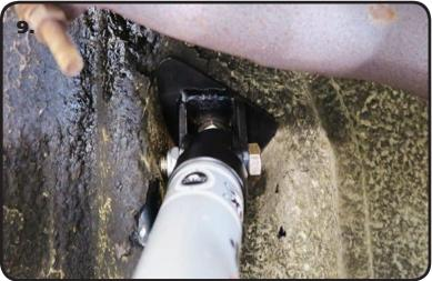
**9.** The Shock is mounted in the Upper Mount with the BODY UP. It is held in place with a 1/2"-20 x 2 1/4" Hex Bolt & 1/2"-20 Nylok. If the threads of the bolt would happen to touch the floor pan of the car, a 1/2" Flat Washer can be installed under the head of the bolt.
