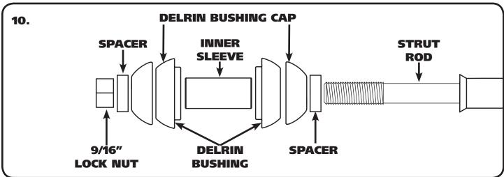
**10**. Install a Spacer on the strut rod followed by the Delrin Bushing Cap. Insert the strut rod through the Bushing Sleeve until the Ball is nested into the Bushing Cap. Install a second Bushing Cap on the strut rod followed by a 2nd Spacer. Next, install a 9/16" Lock Nut on the threads of the strut rod. Install the OEM castle nut on the end of the strut rod with a cotter pin through it.
