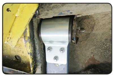
**6.** Swing the Leaf Spring up and attach the **LARGE BUSHING END** of the Composite Leaf Spring into the OEM front leaf spring mount using a 1/2"-13 x 6.5" Hex Bolt and 1/2"-13 Nylok Nut.
