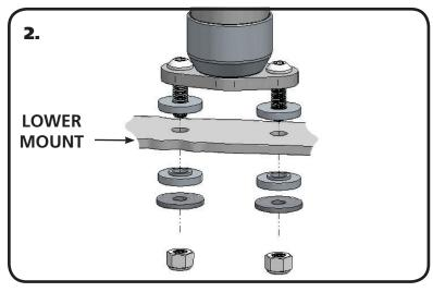
**2. (Figure 2)** shows the assembly of the lower shock bushings. Install a Bushing on the each of threads protruding through the lower shock plates.
