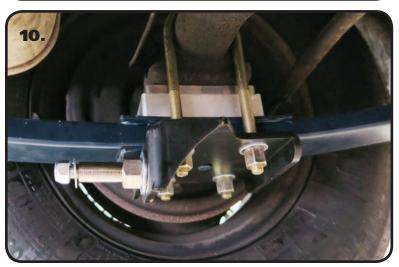
10. The Lower Shock is Bolted to the Lower Shock Mount using the supplied Shock Stud. Install the Studs into the Lower Mounts with a Washer on each side of the Mount. Slide a Washer onto the Stud. Jack the Rear Differential up until the Shocks can be slid onto the Shock Stud. Slide the Shock onto the Stud with the Adjuster Knob pointing inward. Install the supplied 7/ 16" Flat Washer and Nylok Nut onto the Threads and tighten.
