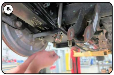
**8.** Install a 5/8" flat washer on each of (4) 5/8"-18 x 7 1/2" hex bolt. Insert the bolt in through the axle mount. Slip the lower leaf spring bracket up onto the U-Bolts WITH THE OFFSET HOLE FORWARD. THE ARROW ON THE BRACKET SHOULD POINT TO THE FRONT OF THE TRUCK. Hold the Leaf Spring Bracket in place and install a 5/8" Flat Washer & 5/8"-18 Nylok Nut on the threads of the u-bolts. Snug the nuts down evenly and tighten them in a criss-cross fashion to 130 ftlbs
