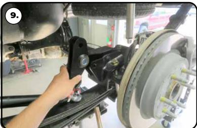
**9.** Insert the pivot/bar into the axle mount. The pivot needs to be installed with the bar mount at the top and the bumpstop to the axle mount.
