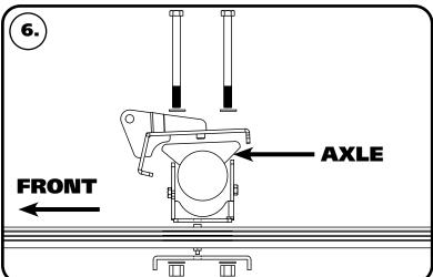
**6.** The traction bar kit uses an upper axle mount and 5/8"-18 x 7.5" hex bolts instead of using the u-bolts that are supplied in the flip kit. The pivot mount will be to the front of the truck with the locating pin nested into the hole of the OEM leaf spring mount.
