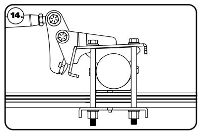
**14.** WITH THE TRUCK ON THE GROUND, THE SET LENGTH OF THE BARS NEED TO BE CHECKED. The bars need to be set so there is approximately 1/8" gap between the bumpstop and axle mount. Adjust the traction bar to get this gap set. After you check the gap, tighten the jam nuts on the traction bar.
