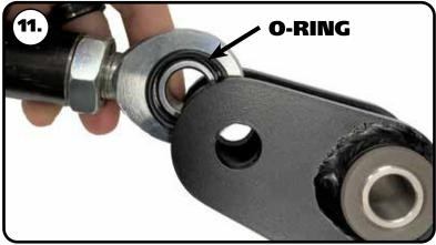
**11.** Install a supplied o-ring on each side of the rod end that will slip into the rear pivot. Hold the o-rings in place as you insert the rod end into the pivot.
