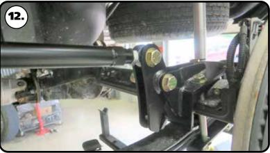
**12.** Insert the rear heim end into the ears of the axle pivot. Align the mounting holes with the through hole of the rod end. Install a 5/8" flat washer on a 5/8"-18 x 2 1/2" bolt. Insert the bolt/washer though the aligned holes. Install a 5/8" flat washer and 5/8"-18 nylok nut on the threads of the bolt. Torque to 115 ft-lbs. Repeat **Steps 3-12** for the other side.
