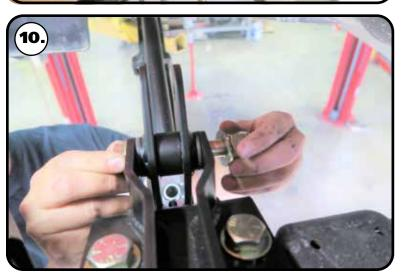
**10.** Install a 5/8" flat washer on a 5/8"-18 x 3 3/4" bolt. With the mounting holes aligned with the pivot inner sleeve, insert the bolt/ washer. Install a 5/8" flat washer & 5/8"-18 nylok nut on the bolt. Torque to 115 ft-lbs.
