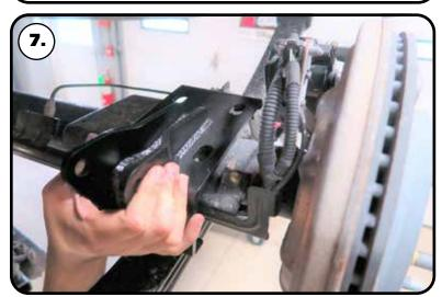
**7.** Sit the axle mount on top of the leaf spring pad with the locating pin nested into the center hole of the leaf spring pad.
