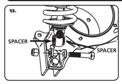
**13.** Install a spacer on each side of the lower Coilover. Slide the shock with the spacers installed into the mount on the lower StrongArm. You may need to jack the rearend up to line up the holes in the bushing with the 1/2" hole in the shock mounts and hold it in place while you install the 1/2" x 2 1/2" bolt and 1/2" Nylok nut. Tighten the upper and lower shock bolts.
