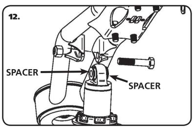
**12.** Install a spacer on each side of the upper Coilover. Slide the assembly into the upper crossmember from the bottom side. If your shock has an adjuster knob position it so that the knob points toward the center of the car. Line up the hole in the spacers with the hole in the upper shock bridge and insert 1/2" x 2 1/2" bolt and install 1/2" Nylok nut.
