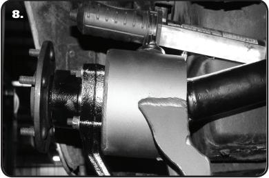
**8.** Install the Knurled Studs into the Trailing Arms. Install the OEM Hub Assembly using (4) 3/8" SAE Nylok Nuts. The Drivers side Trailing Arm has the Shock Mount pointing down and facing the inside of the car. Do this for both sides.
