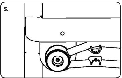
**5.** Refer to Images 5 & 6 for installation of the Crossmember. Apply Loctite to the 7/16"-14 x 3" Stud(1), thread it into the frame approximately 3/4". Slide the Crossmember(A) onto the Studs, holding it in place. Install a 7/16" Grade 8 Flat Washer(2) followed by a 7/16"-14 Grade 8 Regular Nut(3). Do this for both studs. Torque the Nuts to 50ftlbs.
