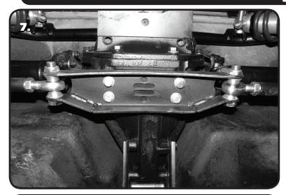
**7.** Install the Strut Rod Bracket onto the bottom of the OEM Center Section with the FLAT side to the rear of the car. Attach the bracket with (4) 3/8" x 1" Hex Bolts, (4) 3/8" SAE Flatwashers, and (4) 3/8" Split Lock washers.
