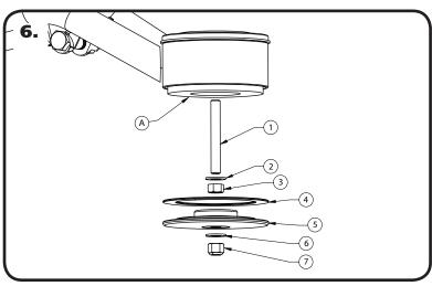
**6.** Install the Isolator Ring onto the Bushing Retainer. There is an area on the retainer that the isolator sits. With the Crossmember in place and the Nuts torqued, slide the Aluminum Bushing Retainer/Isolator on the Stud. Next, install a 7/16" Grade 8 Flat Washer(6) followed by a 7/16"-14 Grade 8 Nylok Nut(7). Do this for both sides. Torque the Nuts to 50ftlbs.
