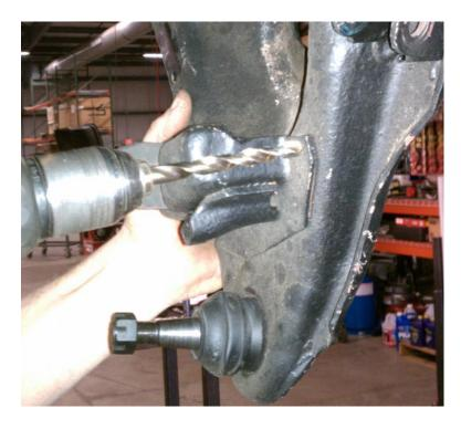
5. Use a drill to drill the spot welds out of the OEM bumpstop/steering stop. Just drill through the mount. Do NOT drill through the control arm. We recommend cleaning the area up after removing it and paint it to keep the area from rusting.
