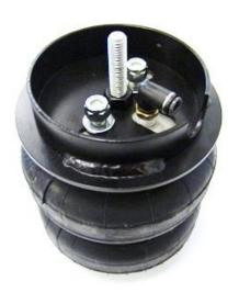
3. Apply thread sealant to a 90 degree air fitting and screw it into the top of the air spring.
