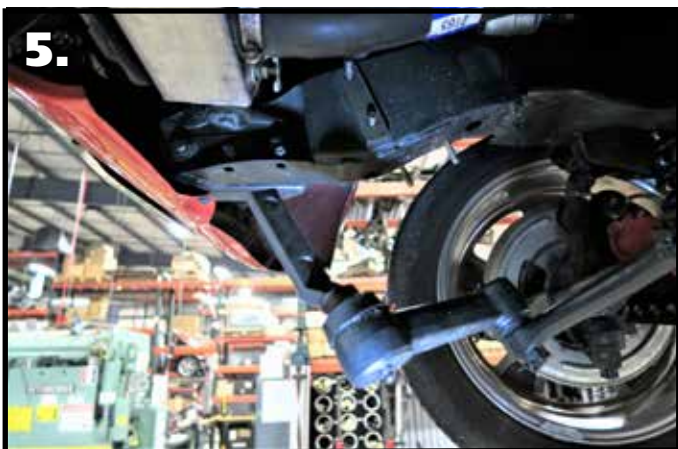
5. Disconnect the idler arms from the frame.
