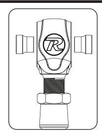
New R-Joints will be quite stiff (75-90 in/lbs breakaway torque) until they "break in" after a few miles of use. After the break in period they will move much more freely. Because the composite bearing race contains self lubricating ingredients, no additional lubrication is needed or desired. Any additional lubrication will only serve to attract more dirt and debris to the R-Joint and actually shorten its life.
