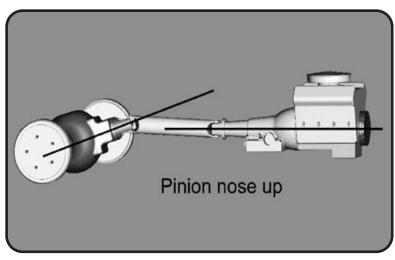
How do you set the pinion angle? On a single-piece shaft you want to set it up where a line drawn through the center of the engine crankshaft or output shaft of the transmission and a line drawn through the center of the pinion are parallel to each other but not the same line.
