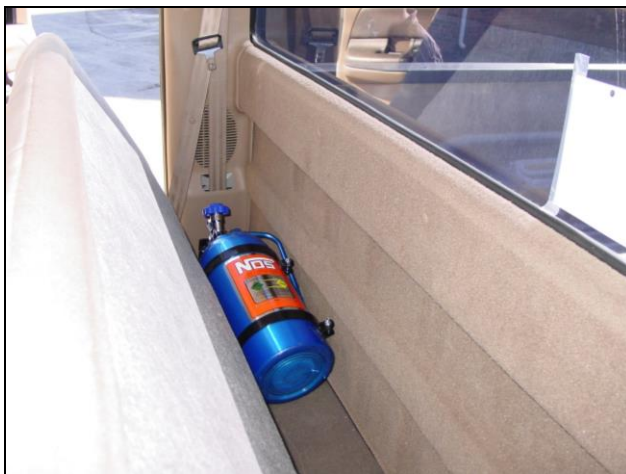
Figure 4 Bottle with blow down tube installed
