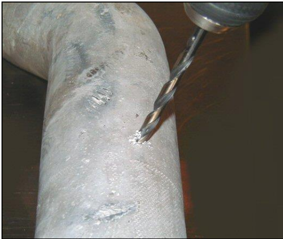
Figure 6 Drill using a 1/4 inch bit.
