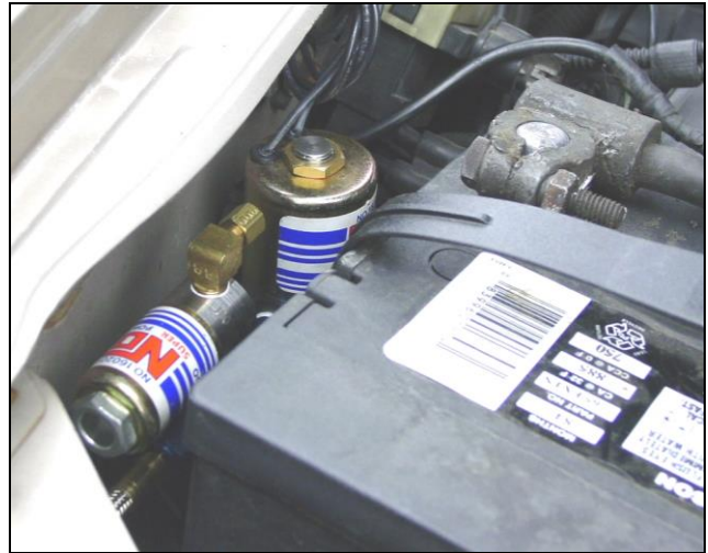
Figure 11 Completed solenoid mounting
