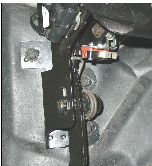
Figure 16 Microswitch in completed location
