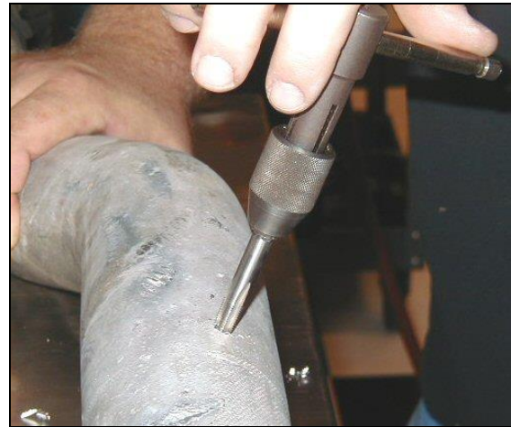
Figure 7 Tap with supplied 1/16 NPT tap.
