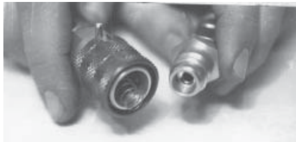
The two parts of the assembly are separated, with the jet in the end cap on the right, the jet is merely dropped out and the new one is inserted
