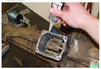
3. Apply a 1/8" bead of RTV silicone sealant around the shifter mount pad, circling the bolt holes.
