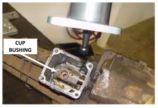
4. Place the shifter's cup bushing into the offset lever. Then guide the shift rod ball into the bushing and place the shifter (1) on the pad.
