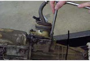
1. Put the transmission in NEUTRAL. Remove the four shifter bolts. Use a suitable knife to break the sealant bond between the shifter and the mount pad, then remove the shifter
