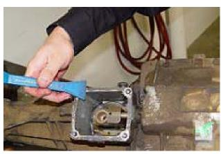
Scrape old sealant from the shifter mount pad, then wipe with brake cleaner. NOTE: Work carefully to prevent any debris from falling into the transmission.
