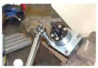
5. Reinstall the shifter bolts and tighten evenly to 12-15 ft-lbs torque.
