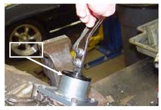
6. Apply a drop of thread locking compound to each screw (2). Then use the screws and lockwashers (3) to assemble your Hurst stick (see page 3) to the shifter, crushing the washers completely. NOTE: The lockwashers are single-use only; replace them if the stick is ever removed from the shifter.
