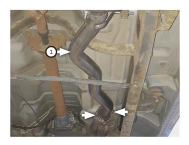
10. Place clamp (4) onto muffler (2) then connect it to inlet pipe. Tighten clamp just enough to allow for adjustment then place (x2) clamps (5) onto muffler outlets.
