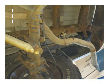
4. Support muffler and disassemble remaining wire hanger from isolator. Then remove and retain (x2) fasteners at muffler to catalytic flange connection and remove exhaust system.
