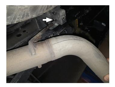
4. Remove bolts and nuts (x4 ea.) from inlet pipe flanges. Then remove bolts (x2) and wire hanger mount to disassemble exhaust system from vehicle. Retain all bolts and nuts for later use.
