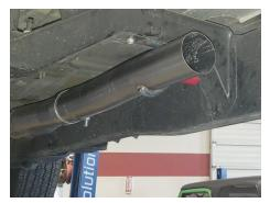
8. Place (x2) clamps (8) onto both ends of muffler (4) then connect it to extension pipe. Tighten front clamp enough to allow for adjustment.
