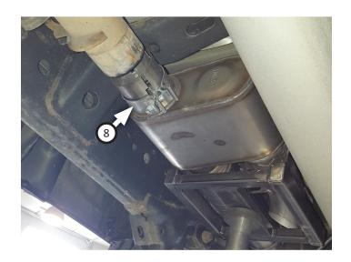
11. Transfer isolators from factory muffler to direct fit muffler hangers to secure it in place. Then clip grounding wire to hanger wire as shown.
