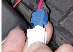
21. Open fuse holder cap, plug in **micro fuse (16)**, then replace cap.
