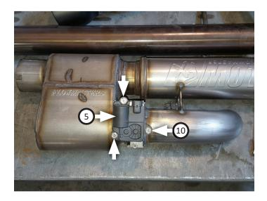
Place clamp (8) onto muffler inlet then connect it to factory inlet exhaust pipe, lining inlet pipe notch up to front pipe tab. Tighten clamp just enough to allow for adjustment.
