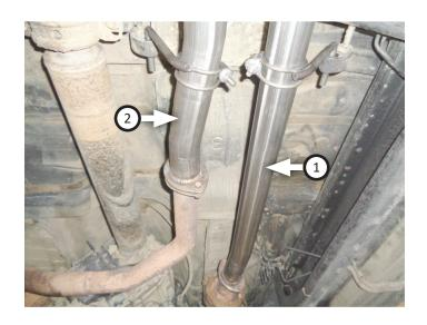
8. Place **left (6)** and **right (5) inlet pipe clamp hangers** onto inlet pipes then insert them into isolators. Tighten clamps enough to allow for later adjustment.
