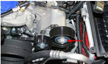
68. Install the smooth idler pulley to the upper water pump provision and the smaller grooved idler to the lower water pump provision. Torque both bolts to 22 ft-lbs.
