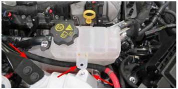
40. Using a panel puller, remove the engine harness from the support bracket located on the passenger side valve cover.
