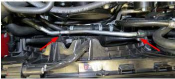
37. Remove two (2) bolts securing the electric fan to the radiator using a 10mm socket. Carefully remove the electric fan assembly.
