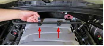
19. Using a deep 10mm socket, remove four (4) bolts securing the manifold cover. Unplug MAP sensor, and cut ties holding the harness to the intake. Do NOT damage the harness.
