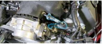
21. Remove the EVAP line from the hardline located on the firewall and from the EVAP solenoid.
