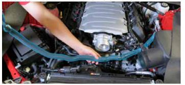
17. Disconnect the electronic throttle body connector from the throttle body.
