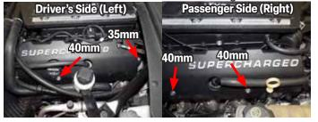
114. Verify no hoses were pinched during installation of the coil covers. Re-position as needed.
