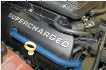
116. Connect driver side pcv hose through the hole in the coil cover.
