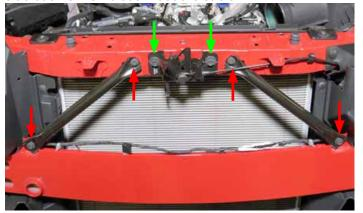
86. Disconnect and remove the horn assembly from the crash beam using a 10mm socket. Using a panel puller, remove the push pins securing the wire harness to the crash beam as well as the radiator shrouds.
