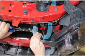
97. Using a 3/4" hose clamp from Bag #2, secure the LTR to Water Pump hose to the bottom LTR barb. Route the hose through the center opening of the radiator shroud.
