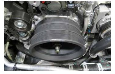
51. Using a 24mm socket and a torque wrench, install the used factory balancer bolt and torque it to 240 ft-lbs. Then remove the factory balancer bolt and discard.
