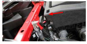
124. Route the EVAP connectors on the supplied water pump harness towards the EVAP solenoid. Install the water pump harness in-between the mating connectors on the EVAP solenoid and factory harness. TIP: Note connector orientation...
