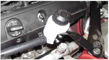
99. Route the LTR to Manifold hose through the hole in the radiator shroud and back towards the manifold. Using a 3/4" hose clamp from Bag #2, secure the hose to the upper barb of the LTR.
