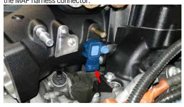
78. If equipped with the MAP adapter/hose assembly, install the long end of the nose, the short fitting end to the brake booster extender, and insert the factory MAP sensor and adapter into the short, straight hose end. Secure the sensor adapter with the suppplied hose clamp.
