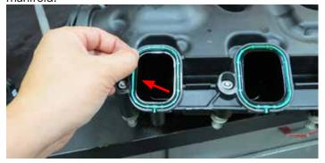
72. Clean and inspect the O-ring gaskets. Replace torn or damage O-rings as needed. Using a razor blade remove the tips off all eight (8) factory O-ring gaskets.
