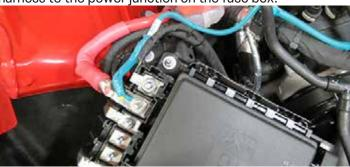
123. Remove the factory GROUND terminal nut attached to the chassis. Attached the GROUND connector on the water pump harness to the chassis ground and secure with the factory terminal nut. Remove the nuts securing the fuse box to the chassis. Gently remove the fuse box from the mounting studs and secure the relay to the mounting stud. Reinstall fuse box nuts.
