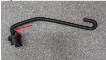
59. Install the supplied water pump isolator onto the water pump noting the orientation.
