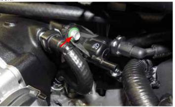
81. Connect the Valley to Inlet hose to the fitting located on the valley cover, to the manifold inlet.
