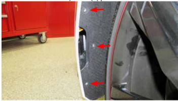
5. Use a 7mm socket to remove six (6) screws securing the corner of the fascia to the fender; three (3) per side.
