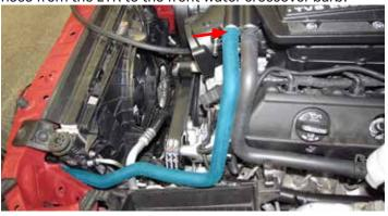
98. Using a 3/4" hose clamp from Bag #2, secure the LTR to Water Pump hose to the outlet barb of the water pump.
