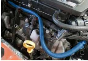
112. Connect the TMAP harness to the TMAP sensor located on the driver side of the manifold.
