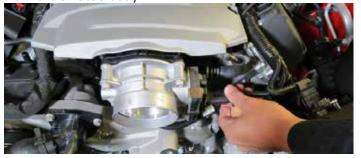
18. Unclip the fuel line from the top of the manifold.
