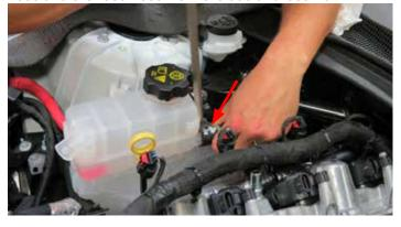
39. Using a deep 10mm socket, remove three (3) nuts securing the coolant reservoir tank. Remove reservoir and set aside.
