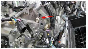
64. Install the supplied tensioner bracket to the provisions on the cylinder head and engine block using two (2) M10 x 100mm bolts and two (2) M8 x 55mm bolts supplied in hardware Bag #1. Torque M10 bolts to 32 ft-lbs and M8 bolts 22 ft-lbs.
