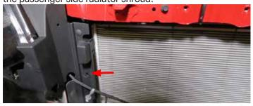
92. Using a panel puller, remove both inner push pins securing the right and left air ducts.
