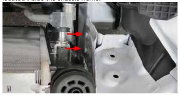
61. Install the water pump assembly onto the water pump bracket. Using the washers from hardware Bag #2 and the factory chassis bolts, mount the water pump bracket to the frame in the location where the chassis bolts were removed. TIP: A secondary wrench may be required to hold the nut located inside the chassis frame.
