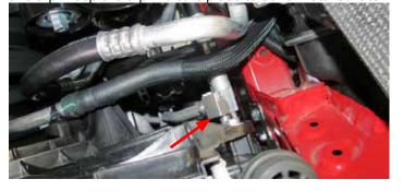
36. Using a panel puller, remove the coolant lines from the fan shroud.
