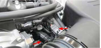
120. Using the supplied worm clamps, secure the inlet elbow to the throttle body and the air intake box.
