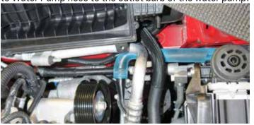
101. Using two (2) 3/4" hose clamps from hardware Bag #2, secure the Surge Tank to Manifold hose to the surge tank and rear water cross over barb.
