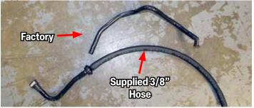
109. Connect the guick-connector on the brake booster hose assembly to the junction on the driver side strut tower. Connect the other end of the hose onto the barb on the supercharger inlet.
