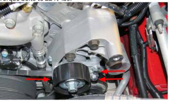
67. Install the larger grooved idler pulley to the FEAD bracket. Torque bolt to 22 ft-lbs.
