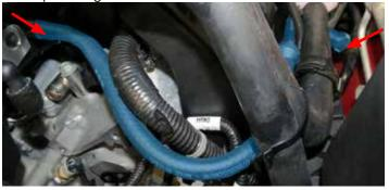
110. Connect the supplied EVAP hose to the hardline on the firewall at the rear passenger side of the manifold. Route the hose along the driver side of the manifold, beneath the coil wires, and connect it to the EVAP solenoid.
