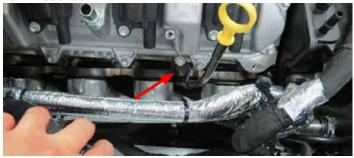
45. Remove five (5) bolts securing the passenger side exhaust manifold to the cylinder head. Carefully remove the exhaust manifold along with the dipstick. Discard the exhaust manifold gasket.
