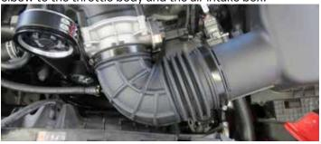
121. Using a razor blade or equivalent, remove the 90° fitting from the factory air inlet PCV hose. Connect the fitting to the supplied air inlet PCV and attach the straight quick connect to the air inlet and the 90° quick connect to the center PCV junction.
