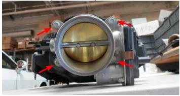
84. Using the supplied gasket and four (4) M6 x 40mm hex flange bolts from Bag #3, secure the throttle body to the supercharger inlet. Reconnect the electronic throttle body connector to the throttle body.
