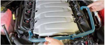
15. Using a 10mm socket, remove the nut securing the noise generator to the firewall.
