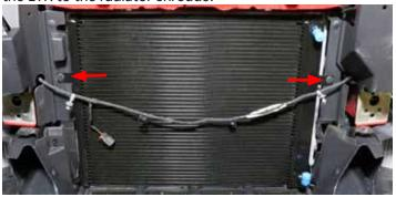
95. Secure the lower portion of the LTR to the air ducts using two (2) M6 x 16mm bolts and two (2) M6 locknuts from hardware Bag #2.
