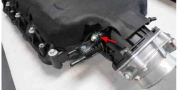
80. Apply O-ring lube to the O-ring on the EVAP solenoid and install EVAP port using the factory EVAP solenoid bolt.
