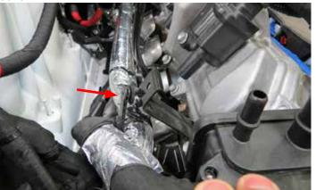
41. Using a 10mm socket, remove the engine harness support bracket. This bracket will not be reused.
