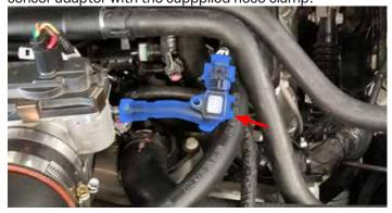
79. Using a 10mm socket, remove the EVAP solenoid from the stock manifold. Inspect the O-ring gasket and replace if needed.
