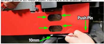
88. Using a panel puller, remove two (2) push pins securing the driver side radiator shroud to the radiator and one securing the rubber shroud. Remove both shrouds. The inner rubber shroud will not be reused.
