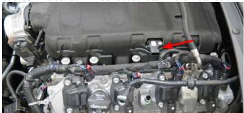
24. Disconnect EVAP connection. Using a 10mm socket, remove ten (10) bolts securing the intake manifold to the cylinder heads. Carefully remove the intake manifold assembly.
