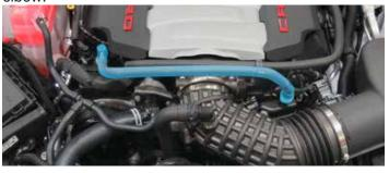
13. Using a hose clamp tool, remove the noise generator hose from the inlet elbow. Loosen the warm clamps securing the inlet elbow and remove the elbow.
