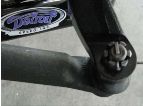
Figure 24 – Attach the Outer Tie Rod to the Steering Arm
