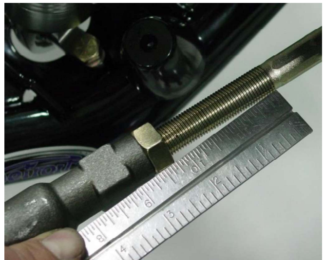
Figure 16 – Measuring the Outer Tie Rods
