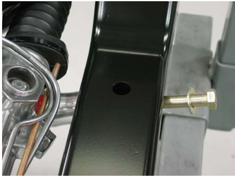
Figure 15 – Attaching the Rack to the Cross Member
