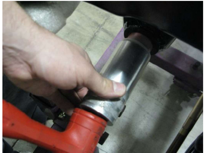
Figure 18 – Fully Installing the Bushings
