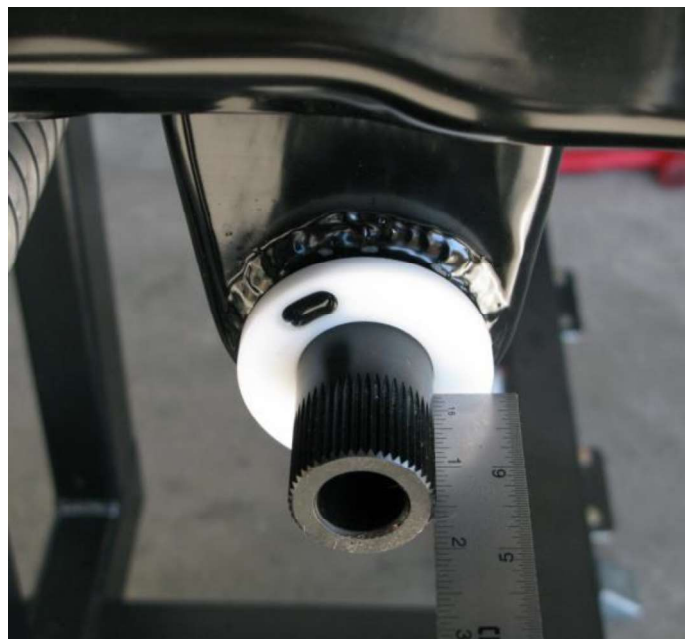
Figure 19 – Measuring the Sway Bar
