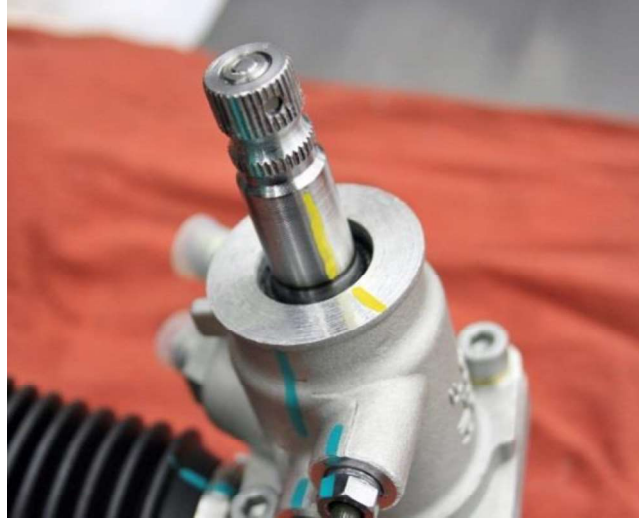
Figure 13 – Center the Rack & Pinion
