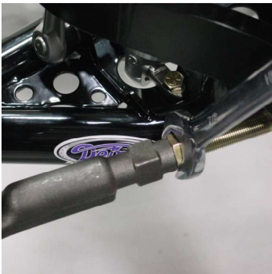
Figure 16 – Measuring the Outer Tie Rods
