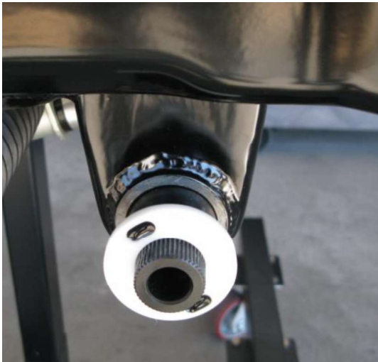
Figure 17 – Installing Bushing & Sway Bar
