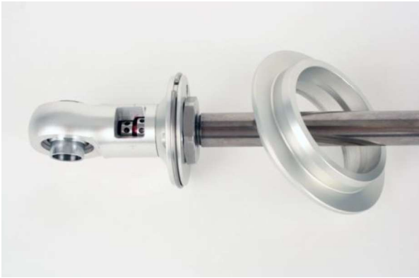
Figure 6 – Removing the Upper Spring Seat
