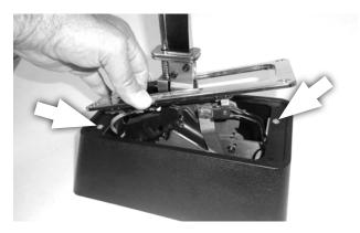
**62.** Secure the tower to the shifter with the two 1/2" flat head Phillips screws.
