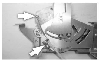
57. Attach the end of the indicator cable to its pin on the shifter with the 1/8" I.D. e-clip. Then attach the cable bracket to the shifter with the two #6 × 1/4" sheet metal screws and #6 washers.
