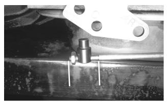
**46.** Thread the swivel onto the cable to about the middle of the threaded section, then reinstall (but do not yet tighten) the jam nut.
