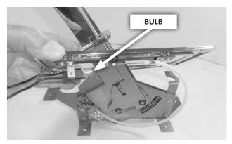
**59. Gently lower the cover assembly over the shifter lever.**Then install the **indicator bulb** in its socket.
