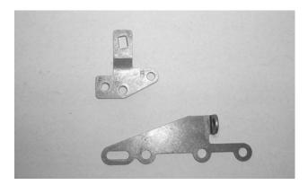
**40. Get the GM selector lever and cable bracket** from the parts kit.
