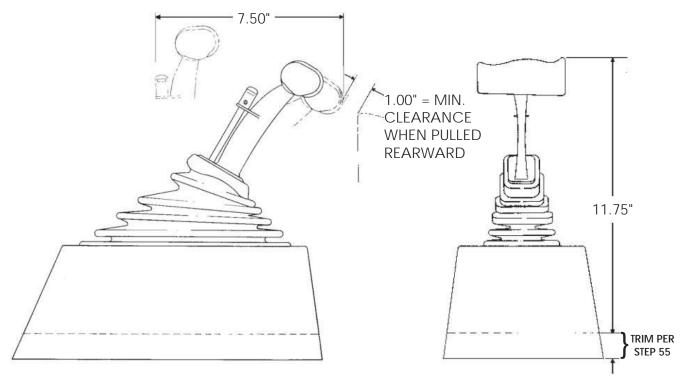
Locate the B&M shifter in your vehicle. Pull the carpet (if any) away from the floorboard where the shifter will be mounted. If the vehicle has a bench seat, move it to the full forward position.
