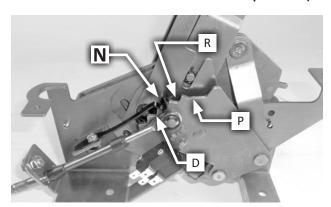
A. With the selector lever still in NEUTRAL (2 clicks from PARK), place the shifter in the NEUTRAL position, and adjust the cable bracket nuts (and swivel, if necessary) until the swivel slips freely in and out of the selector lever hole.
