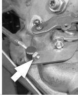
selector lever. Then with the swivel inserted in the selector lever, lightly snug the jam nut.
