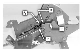
A. On the transmission, manually move the selector lever to the NEUTRAL detent (that is, 2 clicks back from full-forward / PARK). Then in the vehicle, move the shifter to the NEUTRAL position.
