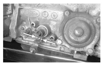
**28.** Move the selector lever to NEUTRAL (2 clicks back from PARK / full forward). If the selector lever points downward, cut it off at the inboard bend, to allow correct positioning of the B&M lever.
