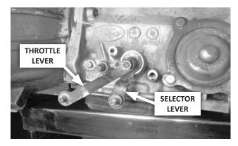
**26. Disconnect stock controls:** Remove and retain the nut and lock washer holding the throttle lever on its shaft. Carefully remove the throttle lever, and move it and its linkage aside, allowing them to hang free. Remove and discard the stock shift linkage.
