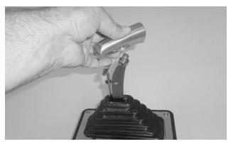
**66.** Carefully thread the T-handle all the way onto the stick.
