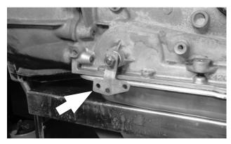
**42. Install the B&M selector lever** using the stock selector lever nut, and tighten the nut to 23 ft-lbs torque. The lever should travel smoothly back and forth, with a positive "click" in each detent.
