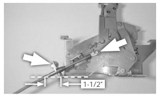
8. Assemble the cable and shifter. Secure the cable eye to the shifter pin with the 1/4" I.D. e-clip. Then secure the cable's mount tab to the outside surface of the shifter base with the 1/4-20 × 1/2" bolt and nut (apply medium strength thread-locking fluid to bolt).
