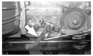
**36.** Reinstall the throttle lever, lock washer and nut on the throttle shaft and tighten securely. The throttle lever must operate smoothly with no binding.
