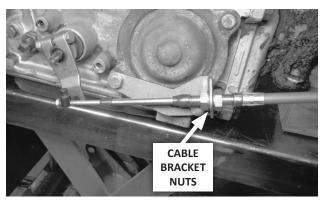
**31.** Attach the shifter cable to the cable bracket: First remove the small jam nut, both plastic dust boots, and one large nut and lock washer, from the cable. Then insert the cable through the cable bracket, reinstall the lock washer and nut (loosely, to allow room for adjustment), and reinstall the dust boots.
