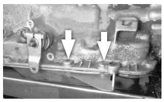
B. <u>C6 transmissions</u>: Install the cable bracket at the two left rear oil pan bolt holes, using the two **5/16-18 × 1"** bolts and flat washers. For stamped sheet-metal (stock) pans, use the two spacers between the pan and bracket. (Spacers are not used with cast aluminum pans.) Tighten the bolts to 12-13 ft-lbs torque.
