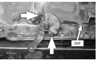
27. If your transmission is equipped with a neutral safety / backup light switch: Remove the two mount bolts and slide the switch off the selector shaft. Cut the wiring harness between the switch and its connector, and discard the switch. (The wires from the connector will be routed to the B&M switches later.)
