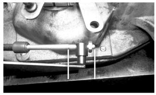
**17.** Thread the swivel onto the cable to about the middle of the threaded section, then reinstall (but do not yet tighten) the jam nut.
