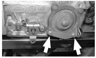
A. <u>C4 / C5 transmissions</u>: Install the <u>cable bracket</u> at the two lower servo cover bolt holes, using the two <u>5/16-18</u> × <u>1" bolts, flat washers</u> and <u>spacers</u>. Tighten the bolts to 12-13 ft-lbs torque.
