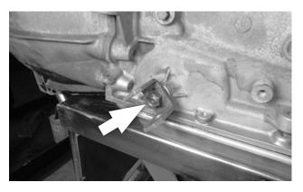
**41. Disconnect stock controls:** Remove and retain the selector lever nut. Remove and discard the selector lever and shift linkage.
