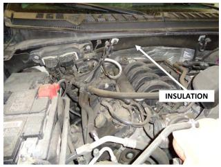
**NOTE:** On some vehicles, the firewall insulation may cover the entire firewall. The adapter can be fastened directly over the insulation, if necessary.
