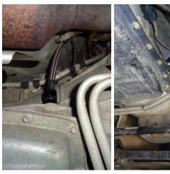
16. Assemble the dipstick tube to the fitting and tighten the nut. **Turn off the vehicle if it is running.**
