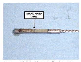
23. Remove B&M dipstick, wipe it off, and reinstall it all the way (knob fully hand tight). Then remove the dipstick again, mark the fluid level with a marker or grease pencil, and turn off the vehicle.
