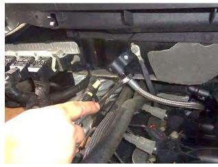
19. Tighten the upper tube nut.
