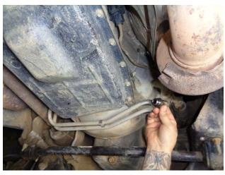
14.Remove the fill cap. If hot (expanded) fluid begins to run out of the port, reinstall the cap, start the vehicle and run it at idle, then remove the cap.
