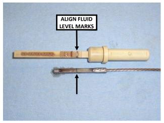
24. Lay the stock and B&M dipsticks next to each other on a bench, and align the two fluid level marks.
