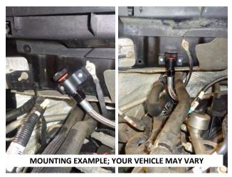
18. Use cable tie(s) to secure the dipstick tube, if required. Fasten the adapter to the chosen location on the firewall using the two self-tapping screws (4).
