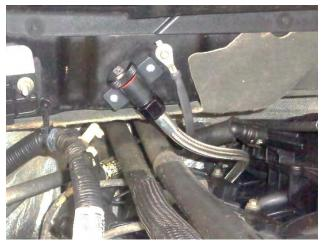
20. Wipe the dipstick and wire with a clean, lint-free rag to remove any rust preventative oil. Then install the dipstick in the tube, and tighten the knob fully hand-tight (until the o-ring is compressed).
