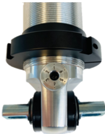
Compression adjustment knobs are located on the bottom mount of RCX coilovers.
