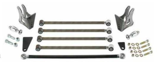
approximately 3/4 of the length of threads. Counting the number of turns assures the bars will be the same length as the other three. It makes no difference whether the rod ends are at the front or the back, but you will have to try each option to find which way works best for your application.
