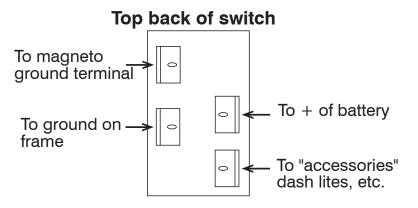
Move switch down to ground mag (kill motor) and shut off accessories. Move switch up to unground mag and turn on accessories.
