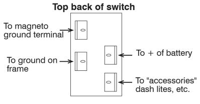
Move switch down to ground mag (kill motor) and shut off accessories. Move switch up to unground mag and turn on accessories.
